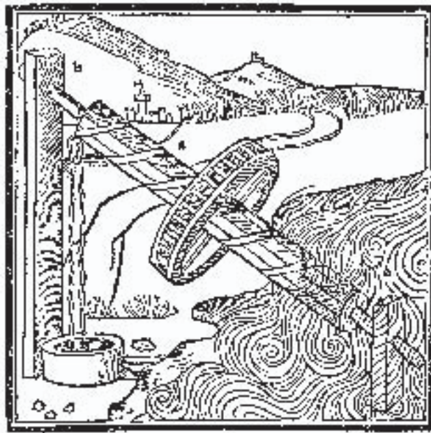
A woodcut of Archimedes' hydraulic screw pump from an edition of Vitruvius's De Architectura published by Fra Giocondo (c.1445-c.1525) in Venice in 1511
